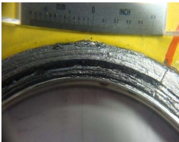
超过1/4圈的填充料丢失 Missing filler more than 1/4 wrap
